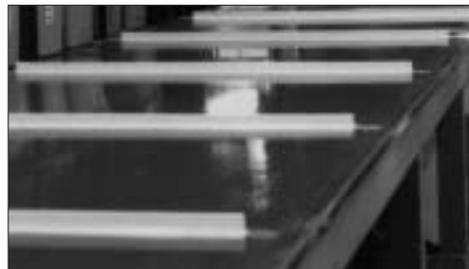
Cleating can be installed on all types of belting.
