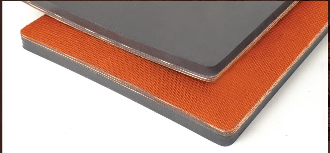
Mulhern Belting's 5-3802 features a strong 3-Ply 600 lbs PIW carcass, a smooth top cover and a bare bottom cover. The stout 3/8" thick top cover is moderately oil resistant and the bare bottom cover makes this a heavy duty slider-bed friendly belt. 3-Ply 600 3/8" x Bare is especially well-suited for the wood industry.
