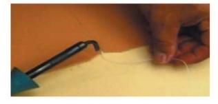
If available, use a soldering iron to seal each end of the pin.
