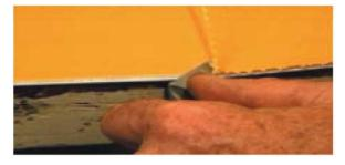
It is critical to keep the edge of the belt perfectly flat while trimming the excess covering to avoid miss-cutting and damaging a spiral necessary for seaming.
