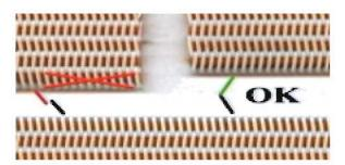
However, it is <u>critical</u> that in determining where to separate, the "good" edge on the second end must align with the "good" edge on the first end. If the spiral to be seamed on the first end points "left", the spiral to be seamed on the second end must point "right", and vice-versa. If the spirals are not properly aligned, you will not be able to make the seam.
